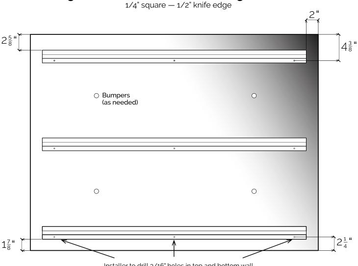
Installer to drill 3/16" holes in top and bottom wall brackets within 2" of end of bracket (max). Other drillings to align with studs whenever possible.
